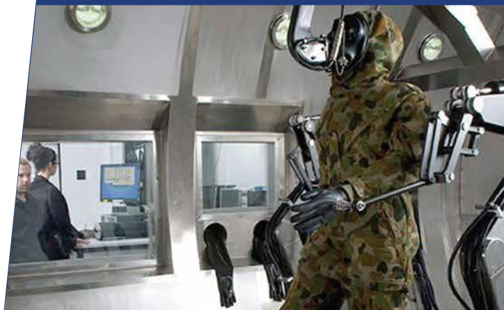
This Environmental Test Chamber & associated equipment was designed, constructed, installed & commissioned by Heuch. The Environmental Test Chamber was featured in a segment of ABC's Catalyst program, presenting the Chambers use as a testing environment for Australian Defence Force uniforms.
